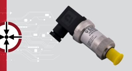
ES Systems has developed a series of medium isolated pressure transmitters suitable for applications with harsh environmental conditions where resistance to corrosive fluids or gases is required. Each sensor integrates a MEMS capacitive pressure sensor die, and a CMOS ASIC for the signal conditioning. The MEMS pressure sensor dies are underpinned by ES Systems' innovative microfabrication process for silicon capacitive sensors.
