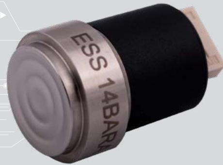
ES Systems has developed a series of pressure sensor modules targeting a variety of markets. Each module integrates an oil filled pressure capsule equipped with a medium isolation diaphragm that protects the MEMS capacitive pressure sensor die. The capsule housing is manufactured from stainless steel. The module can be fitted on a larger housing with a pressure port either by welding or by fitting and O-ring sealing.
